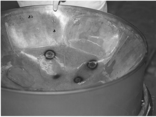
Figure 5 Example of note adjustment by localized heat treatment using a torch.
